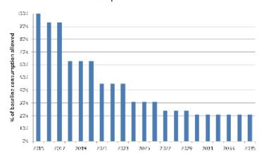
From 2018 onwards, the EU F-Gas Regulation [EU 517/2014] creates massive cuts in the consumption of HFCs in the EU. This reduction scheme, known as the HFC phase-down, is based on a quota system. Quotas are expressed in  $CO_2$  equivalent (kg x GWP).
